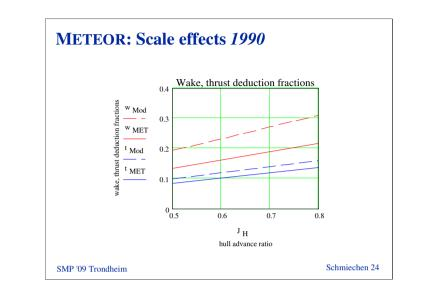
• Results of the full scale tests with the METEOR have been compared with results of corresponding model tests
