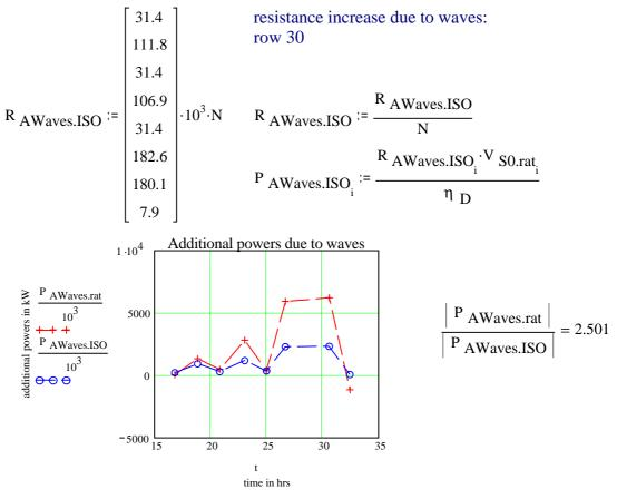
Final performance data according to rational evaluation Reduction to the no-wind and no-wave condition  $V_{S3_i} := (V_{S0.rat_i})^3$  $P_{B0.rat} := A_{req} \cdot X_{req} - P_{AWaves.rat} - P_{AWind.rat} + V_{S3} \cdot X_{req_2}$  **Rates of revolutions**
