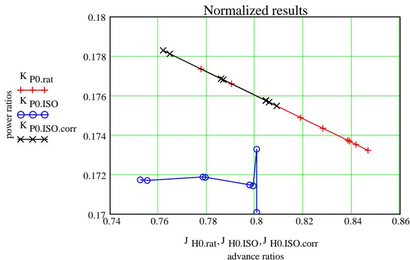
**The differences in magnitude and, particularly, in trend of the normalized results between the proposed rational and the proposed ISO evaluations are due to inconsistencies in the ISO procedure. To cope with them by changing the rates of revolution according to the rational power characteristic is certainly not rational.**
