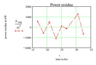
In view of the fact that the scatter of the power values around the propeller power line is very small these large residua indicate that the wave resistance is not correctly assessed by the proposed ISO procedure.
