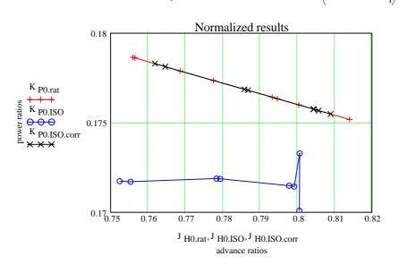
The differences in magnitude and, particularly, in trend of the normalized results between the proposed rational and the proposed ISO evaluations are due to inconsistencies in the ISO procedure. To cope with them by changing the rates of revolution according to the rational power characteristic is certainly not rational.
