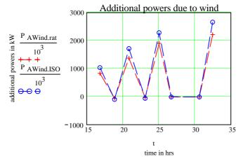
$$\frac{\left|\begin{array}{c} P_{AWind.rat} \\ \end{array}\right|}{\left|\begin{array}{c} P_{AWind.ISO} \end{array}\right|} = 0.825$$
