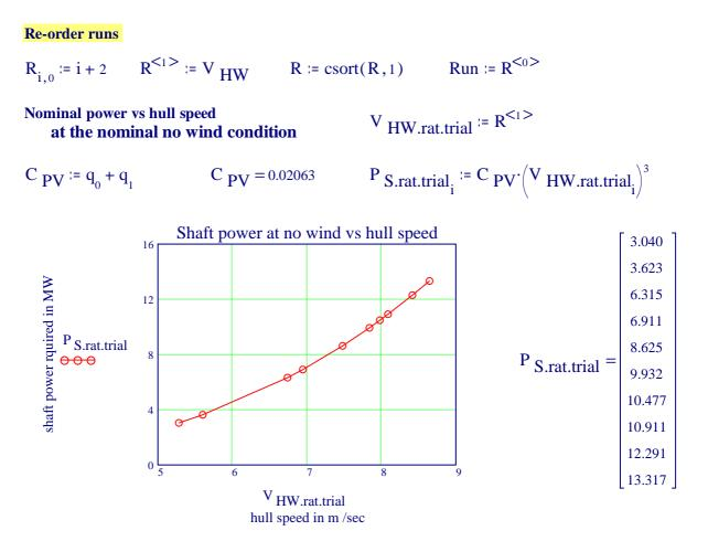
**Nota bene:** The power at the nominal no wind condition identified is that at the hull condition, the loading condition and the sea condition prevailing at the trials!
