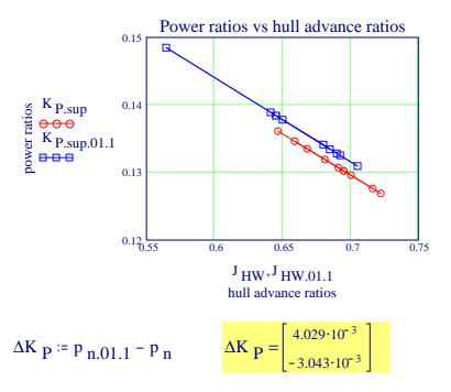
The powering performances in the behind conditon identified fpr both ships are differing only slightly in values.
