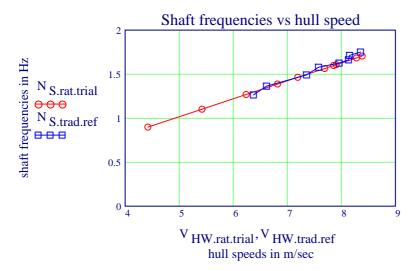
Evidently the results of the rational evaluation at the trials condition, requiring no prior data, and the results of the traditional evaluation at the only slightly different reference condition, requiring very many prior data, last but not least the computed values of the propulsive efficiency, are very nearly the same, not to say 'identical'.
