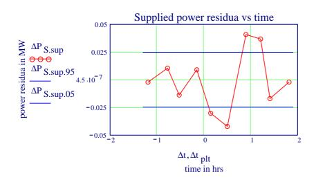
Accordingly the conventions adopted 'describe' the power data perfectly well! The relatively small value of the confidence radius cannot be judged objectively, as the confidence ranges of the mean values have not been provided as in case of the analysis of the ANONYMA trials.
