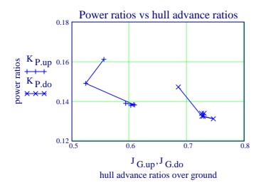
Evidently the values at the first double run are outliers eliminated without further study of possible reasons. In the traditional evaluation the values at the first two double runs, i. e. the first four data sets have been ignored. For ready comparison of results the same data set will be used in PATE\_01.2.
