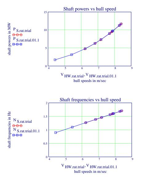
Evidently the final results do not differ for the two different data sets!
