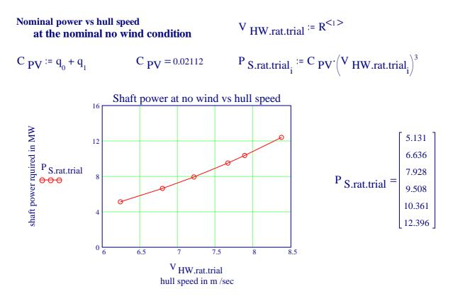
**Nota bene:** The power at the nominal no wind condition identified is that at the hull condition, the loading condition and the sea condition prevailing at the trials!
