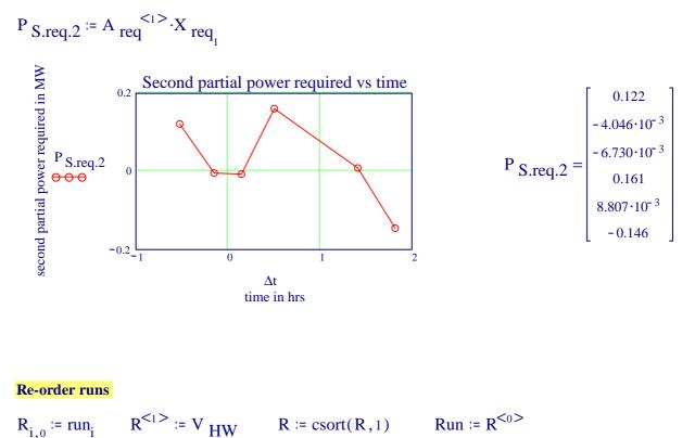
Run number re-ordered according to increasing hull speed through speed The natural count of runs is coveniently reduced by 1!
