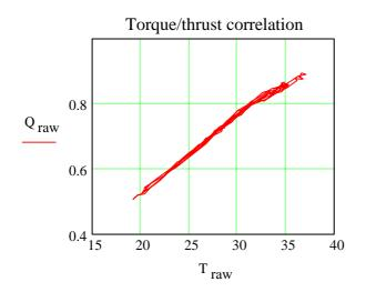
Something has happened in the measurements of the higher torque values? Was there a problem with the dynamometer or did the flow pattern at the model propeller suddenly change?
