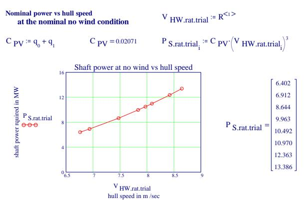
**Nota bene:** The power at the nominal no wind condition identified is that at the hull condition, the loading condition and the sea condition prevailing at the trials!
