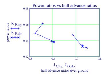
Evidently the values at the first double run are outliers eliminated without further study of possible reasons in PATE\_01.1. In the traditional evaluation the values at the first two double runs, i. e. the first four data sets have been ignored. For ready comparison of results the same data set has been used in PATE\_01.2.
