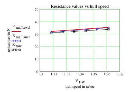
The model resistance identified excluding the measured thrust values is thus nearly identical to the towing resistance.
