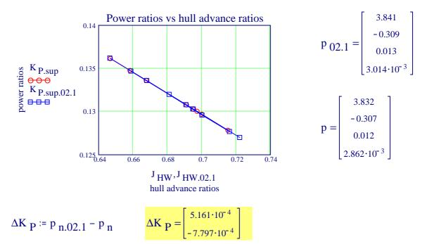
The powering performances in the behind conditon identified for the two different data sets are in perfect agrrement.
