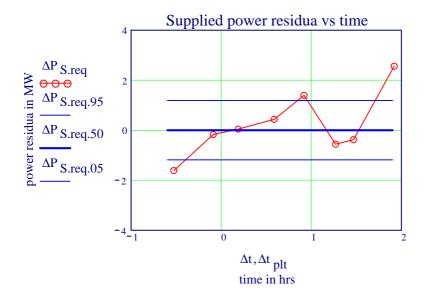
As usual the required power residua are much larger than in case of the supplied power due to the uncertainties in the wind measurements and the crude wave observations.
