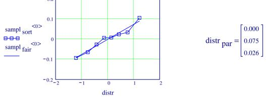
According to the plot of differences in currents identified and the subsequent check of the distribution the differences are 'of cause' not quite normally distributed. Thus the following analysis is not quite justified.
