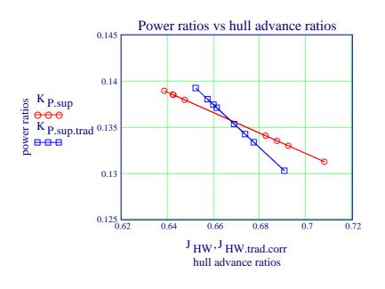
Evidently the power ratios versus the advance ratios identified differ significantly in tendency. There may be many reasons, among them the surface effect due to the extremely small nominal propeller submergence not correctly being accounted for in the undisclosed traditional procedure.
