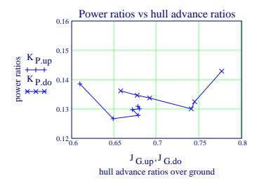
Evidently the values at the first double run are outliers to be eliminated without further study of possible reasons. In the traditional evaluation the values at the first two double runs, i. e. the first four data sets have been ignored.
