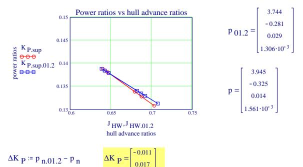
The powering performances in the behind conditon identified for the two different data sets are differing in value and in tendency slightly more than in the case before.
