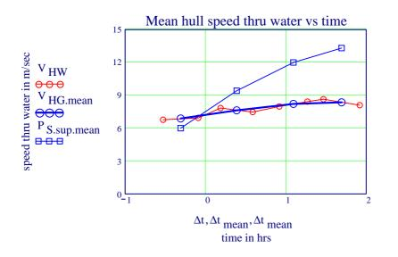
In the present case the mean speed over ground happens to be equal to the speed over ground at the mean time between the two corresponding runs.
