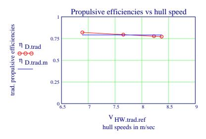
This analysis shows that the traditional evaluation is practically in accordance with the convention, implying that the propeller is permanently operating at the same normalised condition, resulting in the quadratic resistance law.
