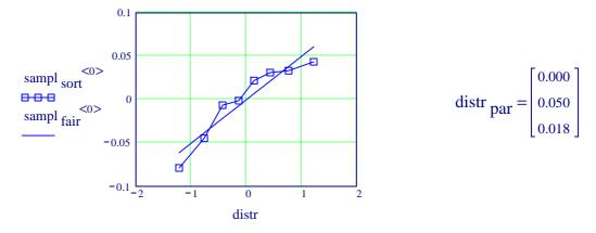
According to the plot of differences in currents identified and the subsequent check of the distribution the differences are not quite normally distributed. Thus the following analysis is not quite justified.
