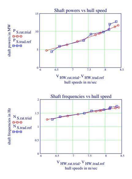
Evidently the results of the rational evaluation at the trials condition, requiring no prior data, and the results of the traditional evaluation at the only slightly different reference condition, requiring very many prior data, last but not least the computed values of the propulsive efficiency, are very nearly the same, not to say 'identical'.
