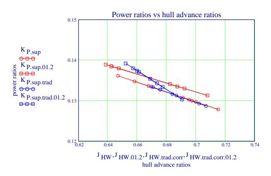
In this case the hull speeds through the water identified differ only very little and thus the powering performance in the behind condition identified by the rational and traditional procedures 'coincide'!
