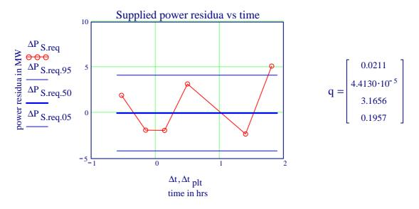
As usual the required power residua are much larger than in case of the supplied power due to the uncertainties in the wind measurements and the crude wave observations.
