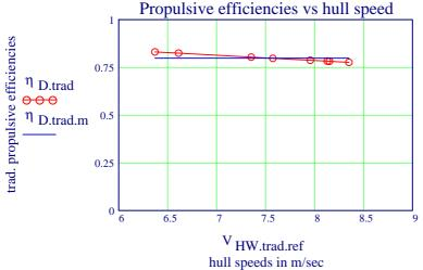
This analysis shows that the traditional evaluation is practically in accordance with the convention, implying that the propeller is permanently operating at the same normalised condition, resulting in the quadratic resistance law.
