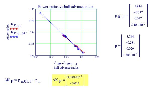
The powering performances in the behind conditon identified for the two different data sets are differing only very slightly in value and in tendency.
