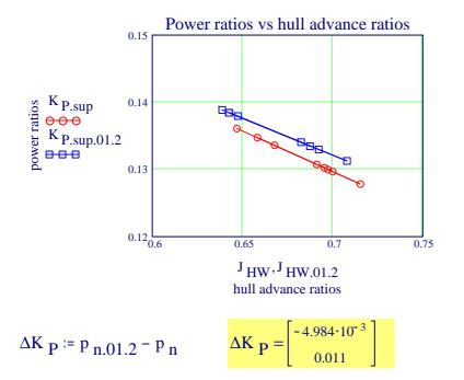
The powering performances in the behind conditon identified for both ships are differing slightly in value and in tendency.
