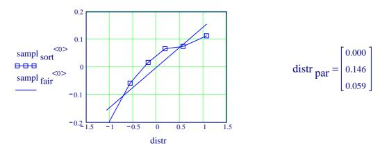
According to the plot of differences in currents identified and the subsequent check of the distribution the differences are 'of cause' not quite normally distributed. Thus the following analysis is not quite justified.
