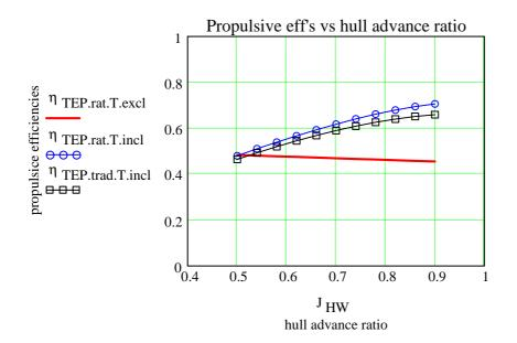
Evidently the results are quite unsatisfactory, the energy balance not accounting for unknown effects of the towing tank environment, e.g. drift due to previous tests and tidal waves.
